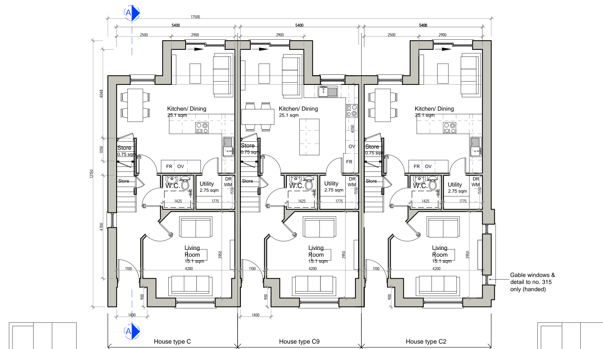
01 Ground Floor Plan Scale 1:100 Terrace Type 'C'/C9/C2' 3 bed Terrace- Ground Floor Plan AREA : Type C - 55.6sqm, Type C9 - 55.6 sqm, Type C2 - 55.6 sqm O/all Area : Type C -108.2sqm / 1164 sq ft, Type C9 -108.2sqm / 1164 sq ft, Type C2 -108.2sqm / 1164 sq ft O/all Excl. stairwell to 1st floor: Type C -105.9sqm/ 1140sqft, Type C9 -105.9 sqm/ 1140sqft, Type C2 -105.9 sqm/ 1140sqft
